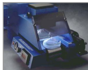
Automated facemask curing
