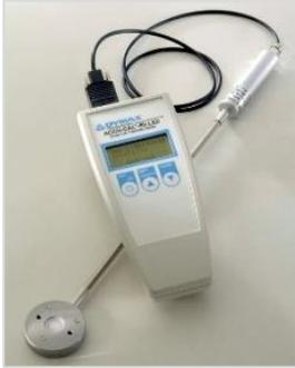
The typical intensity output degradation rate of the unit when run at 100% power and a 100% duty cycle is approximately 8% per 1,000 hours of run time. As with any type of energy source, environmental and operating conditions will have a direct effect on actual degradation rates. Intensity of the BlueWave® MX-250 can be measured with a standard ACCU-CAL™ 50-LED radiometer using flood-lamp intensity mode.
